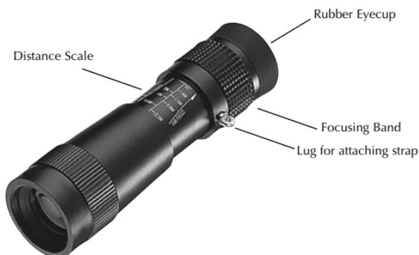
**Using glasses.** To maximize field of view with glasses on, fold the rubber eyecup to the 'down' position - remembering to fold it back up if you or anybody else wants to use the instrument without glasses.
